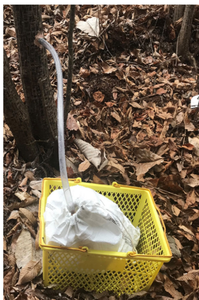
図-1. 樹液採取装置 Fig. 1 Maple sap sampling device
